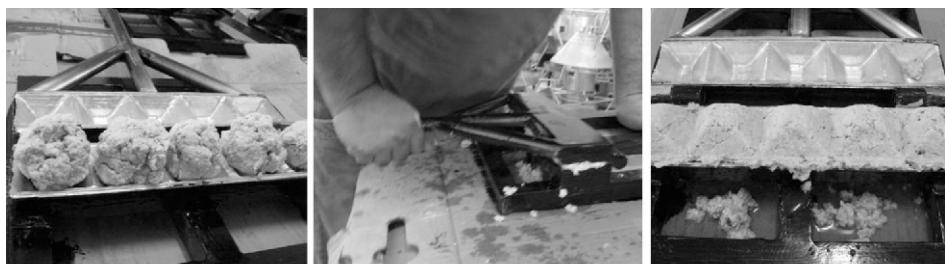
Figure 2. Briquetting of wastes, showing from left to right: placement of balled mixtures in the molder, compaction of the materials, and the pillow-shaped briquettes produced.
