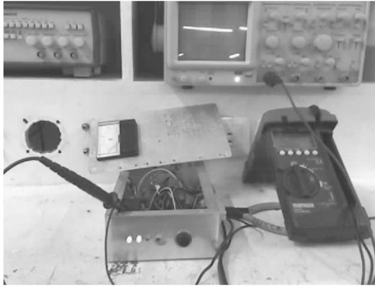
Figure 3. The oscilloscope showing 90% duty cycle with the green and the yellow LEDs lit up indicating trickle charging.
