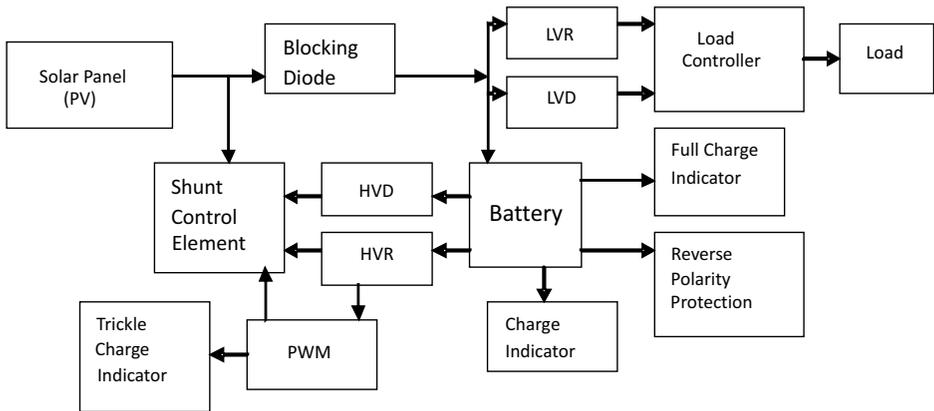
Figure 1. Block diagram of a battery charge-controller
