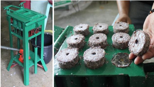
The 15-day actual field production test performed by identified members of UCLA using the same mixtures exhibited an average production rate per day of 105 to 149 briquettes (1.68 to 1.92 kg/hr)). The analyzed data in pcs/hr confirmed the results of the laboratory testing where the number of briquettes produced had no significant difference among the different materials used.
