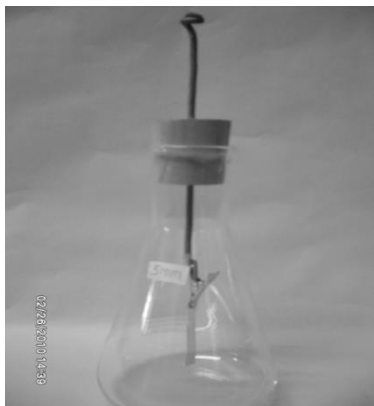
Figure 4. Uncharged electrostatic. The leaves hang straight down together.
