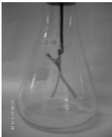
Figure 5. Charged electrostatic. The leaves diverge.
