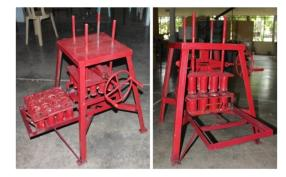
identified members of UCLA using the same mixtures exhibited an average production rate per day of 105 to 149 briguettes (1.68 to 1.92 kg/hr). The analyzed data in pcs/hr confirmed the results of the laboratory testing where the number of briquettes produced had no significant difference data obtained had no significant difference among the different materials used.
